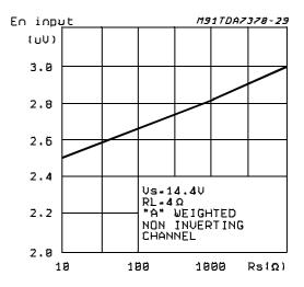
Figure 15: En input vs. R<sub>S</sub> (Single Ended)
