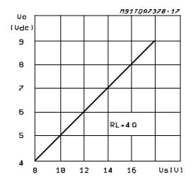
Figure 3: Output Power vs. Supply Voltage (Single Ended)
