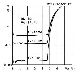
**Figure 7:** Output Power vs. Frequency (Single Ended)
